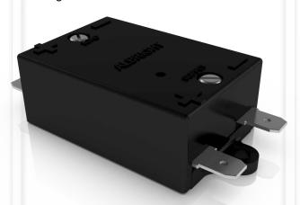
The CC74 module is available in two universal types covering voltages from 12V to 60V and 60V to 96V, where the final output voltage is a fixed ratio of the input voltage. Versions are also available that have a fixed, regulated output voltage. These regulated devices provide the optimum coil voltage without the need for any pre-regulation and can offer the opportunity for customers to use a single type of contactor with different supply voltage systems.
