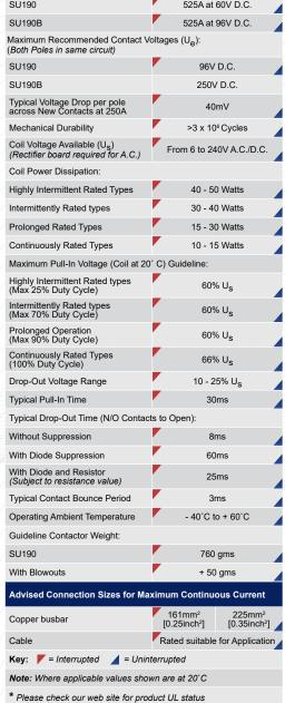
Performance data provided should be used as a guide only. Some from figures may be necessary according to application. Thermal current ratings stated are dependent upon the size of co
