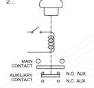
Knob in "ON" position Coil energised Main contacts closed N.O. auxiliary contacts closed
