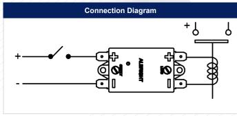
Pulse Width Modulation (PWM) technology is a common technique for coil economising in modern contactor applications. After an initial closing pulse the module regulates the coil down to the specified power dissipation (around 20%).
