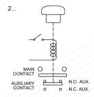
Knob in "ON" position Coil energised Main contacts closed N.O. auxiliary contacts closed
