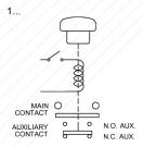
Knob in "ON" position Coil de-energised Main contacts open N.O. auxiliary contacts closed
